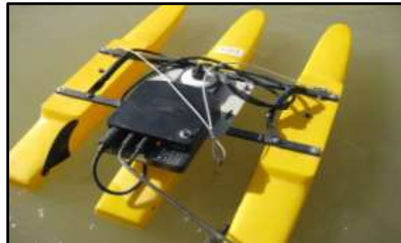
Fig.3: Stream flow measurement using an ADCP Fig.4: SonTek river surveyor ADCP
